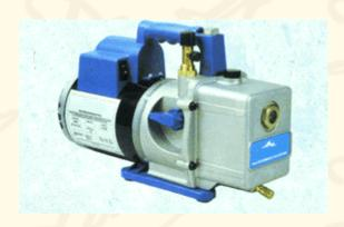
The D9145 Vacuum Pump is a high quality system designed to evacuate air at a rate that is twice as fast as major competition pumps. The heavy duty ½ HP motor's high torque design facilitates easy startup and efficient operation. The two stage design enables the user to pull a deeper ultimate vacuum, and the systems offset rotary vanes builds a powerful compression within the pumping chamber to reduce system pressure.
